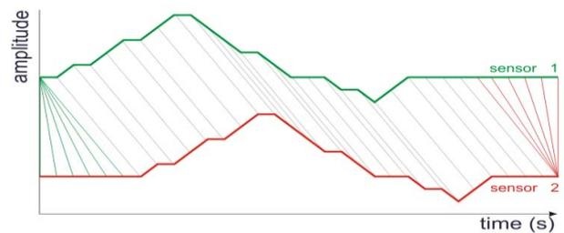
Figure 6: An ideal alignment of two magnetic signals
