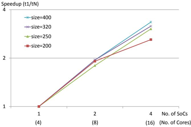
Fig. 3: Strong Scaling for benchmark Dense Matrix Multiplication (Square Matrices). Matrix size varies: 200,250,320,400. Block size is constant and equal to 10. The time used for calculating the speedup accounts for both the User Time and the Kernel Time.
