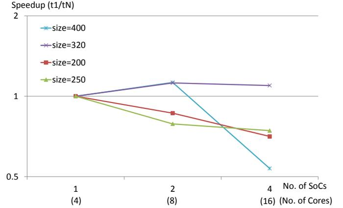
Fig. 4: Weak Scaling for benchmark Dense Matrix Multiplication (Square Matrices). Matrix size varies: 200,250,320,400 on each single SoC (to keep the work almost constant on each core/SoC). Block size is constant and equal to 10. The time used for calculating the speedup only accounts User Time (without Kernel Time).
