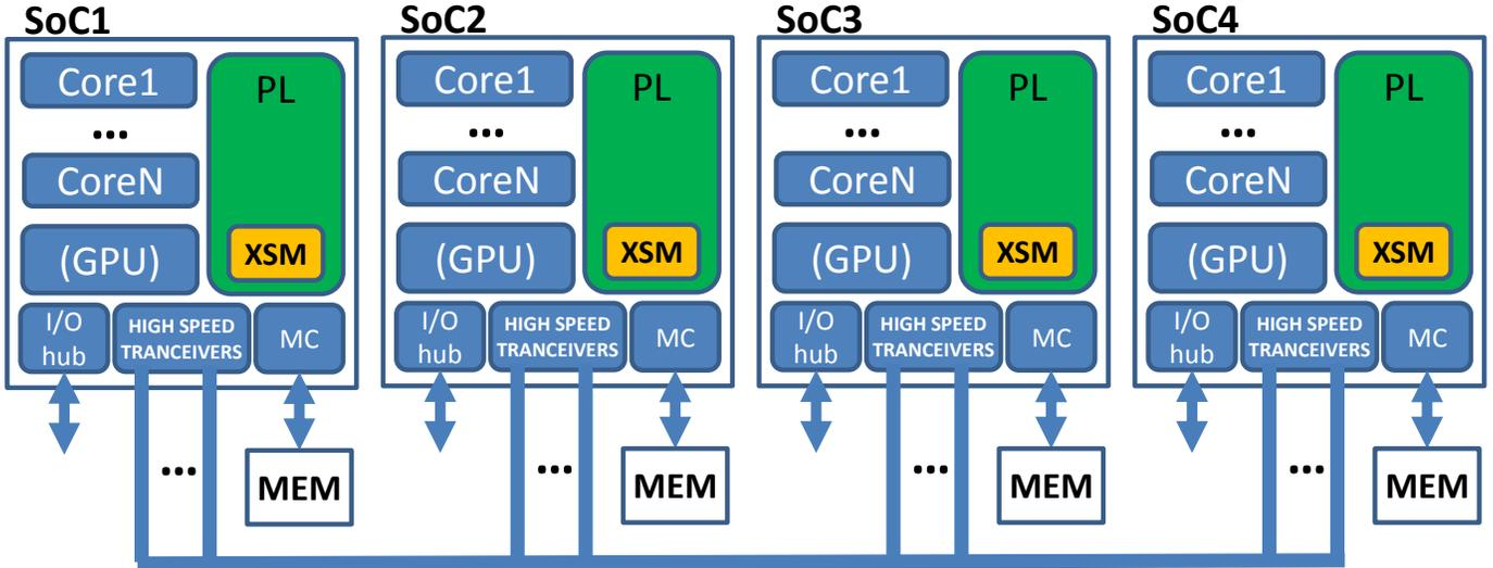
Fig. 1: AXIOM Scalable Architecture. An instance consisting of four boards, each one based on the same System-on-Chip (SoC). GPU is an optional component. MC=Memory Controller. PL=Programmable Logic. XSM=eXtended Shared Memory
