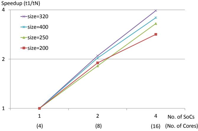
Fig. 2: Strong Scaling for benchmark Dense Matrix Multiplication (Square Matrices). Matrix size varies: 200,250,320,400. Block size is constant and equal to 10. The time used for calculating the speedup accounts only for the User Time (without Kernel Time).
