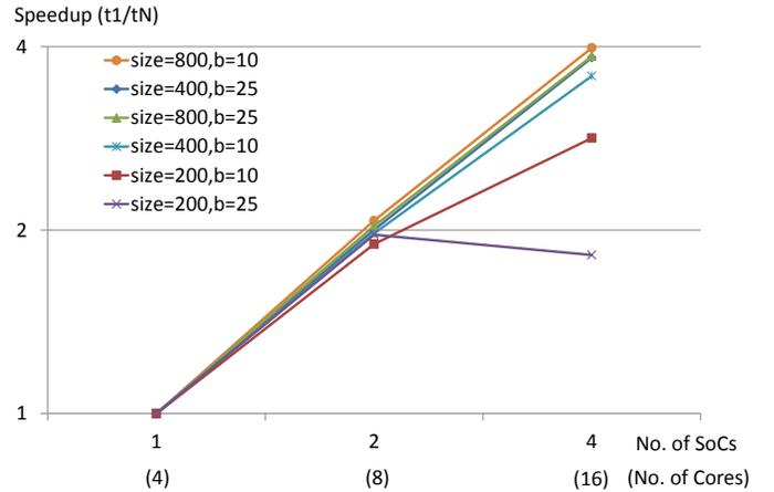
Fig. 5: Effect of the thread granularity (through the block size) on strong scaling for benchmark Dense Matrix Multiplication (Square Matrices). Matrix size varies: 200,250,320,400. Block size assumes values 10 and 25. The time used for calculating the speedup accounts only for the User Time (without Kernel Time).
